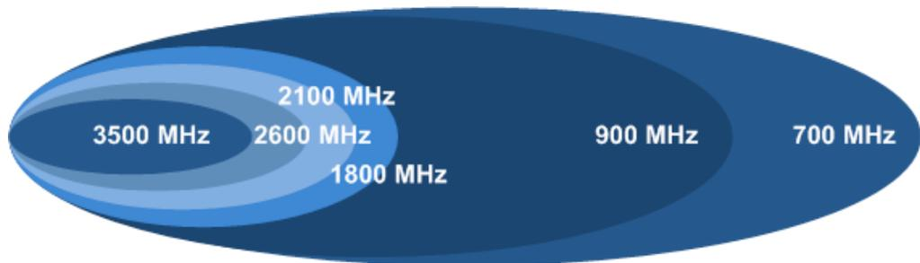
Figure 2 Coverage distance for different spectrum bands.
