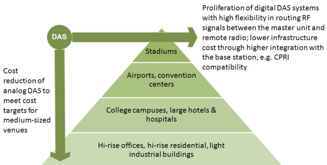
Figure 9 Evolution of DAS to reduce cost for large venues and to scale service into smaller venues.
