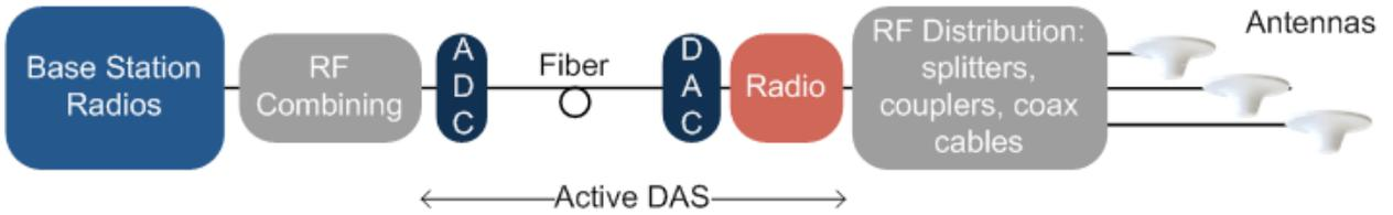
Figure 4 Active distributed antenna system.
