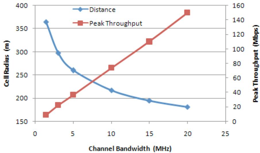
Figure 1 Distance and peak throughput performance for 2x2 MIMO LTE micro cell in urban clutter.
