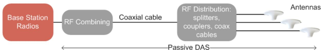
Figure 3 Passive distributed antenna system.
