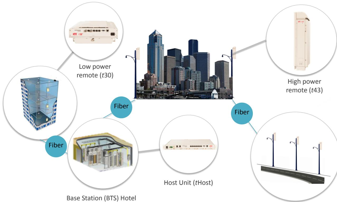
Figure 1 Dali RF Router™ consists of the tHost master hub and t30 and t43 remote radios.
