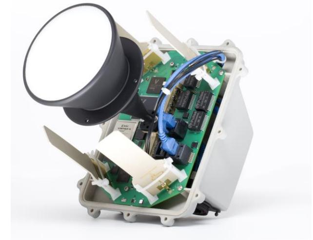
**Figure 2.** HaulPass micro SC 5/60 GHz small cell wireless backhaul system. Antennas are fixed. Source: VubIQ
