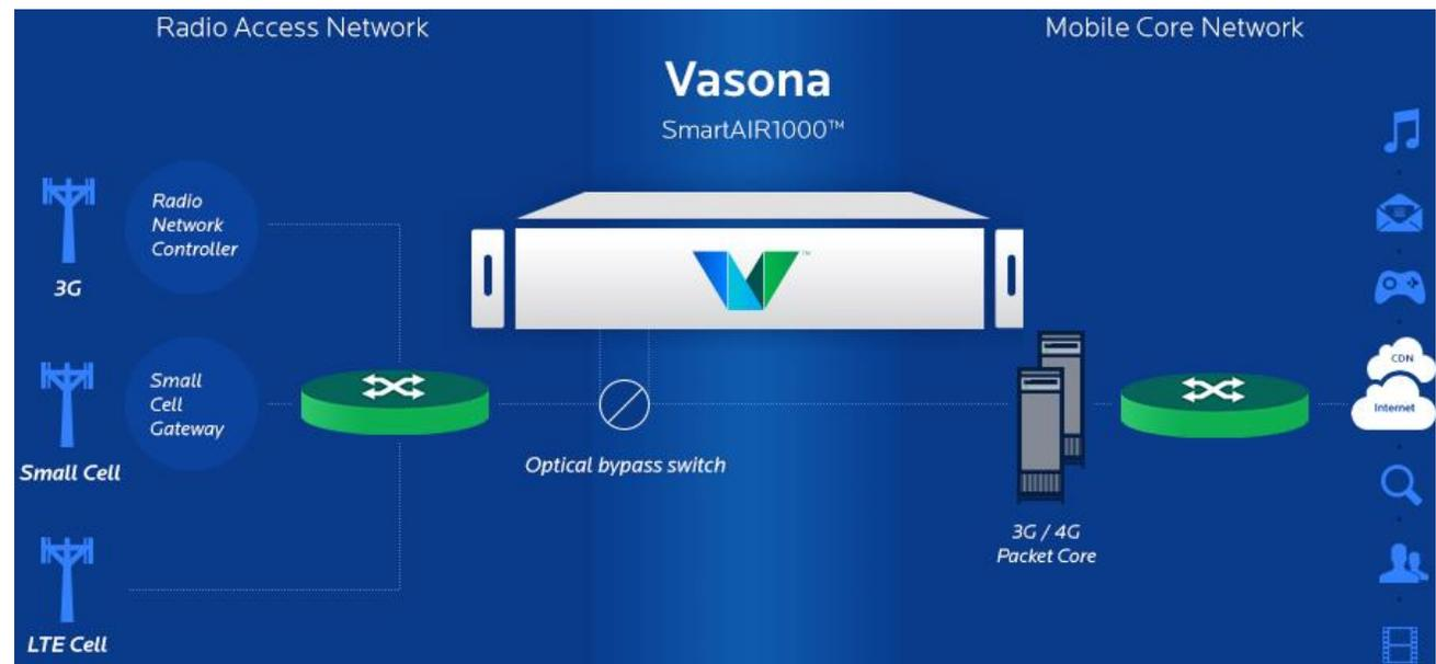
**Figure 2. The Vasona SmartAIR1000™ deploys between the RAN and the mobile core network.**
