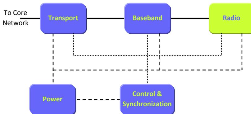
**FIGURE 3 BASE STATION LOGICAL ARCHITECTURE.**
