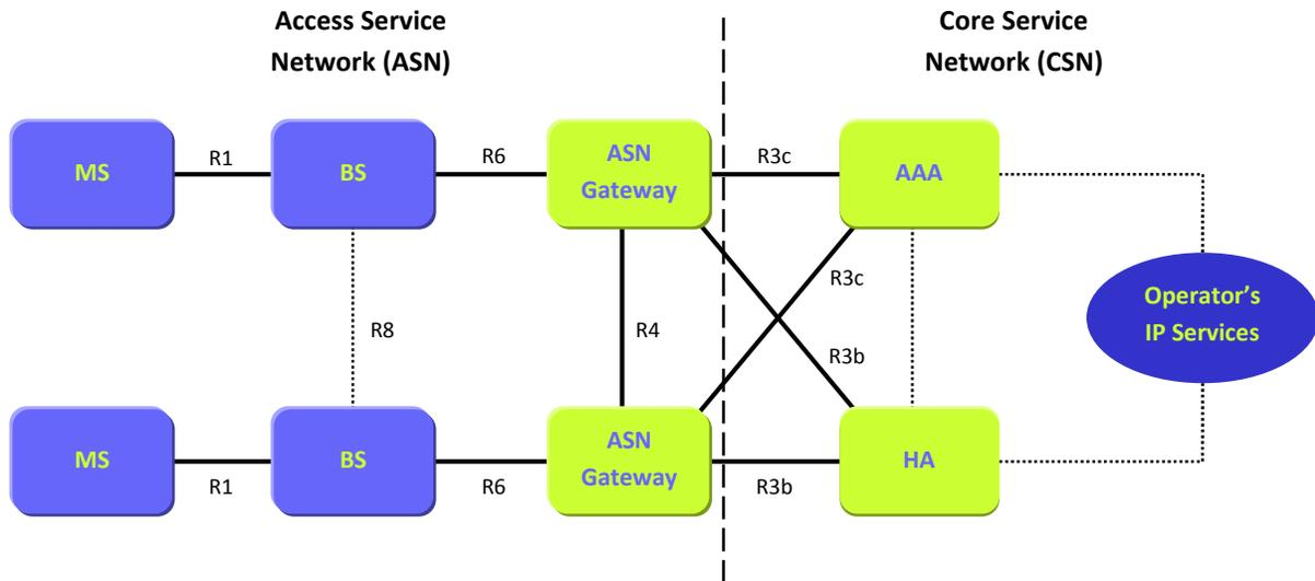
**FIGURE 2 WIMAX NETWORK REFERENCE MODEL.**
